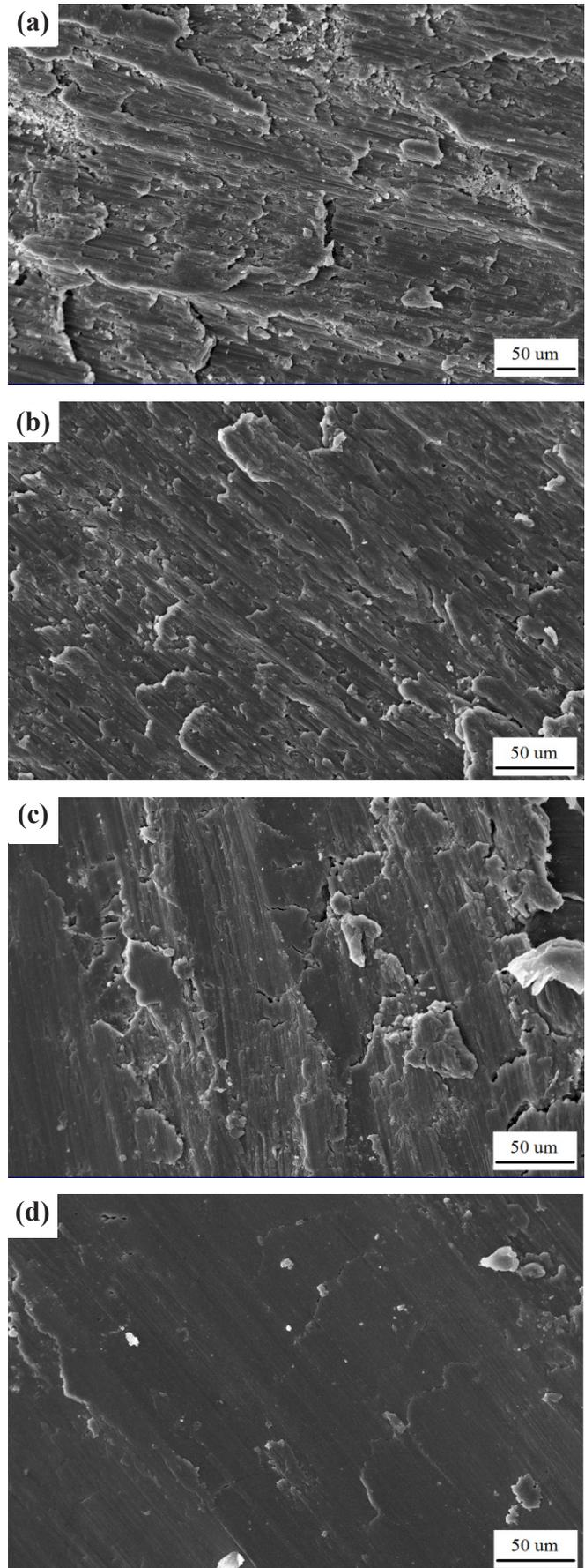
Fig. 6. SEM micrographs from the worn surface of the specimens, (a) A356/(ZrSiO<sub>4</sub>)<sub>p</sub>-LL, (b) A356/(ZrSiO<sub>4</sub>)<sub>p</sub>-SL, (c) A356/(Al-ZrSiO<sub>4</sub>)<sub>cp</sub>-LL, and (d) A356/(Al-ZrSiO<sub>4</sub>)<sub>cp</sub>-SL.
