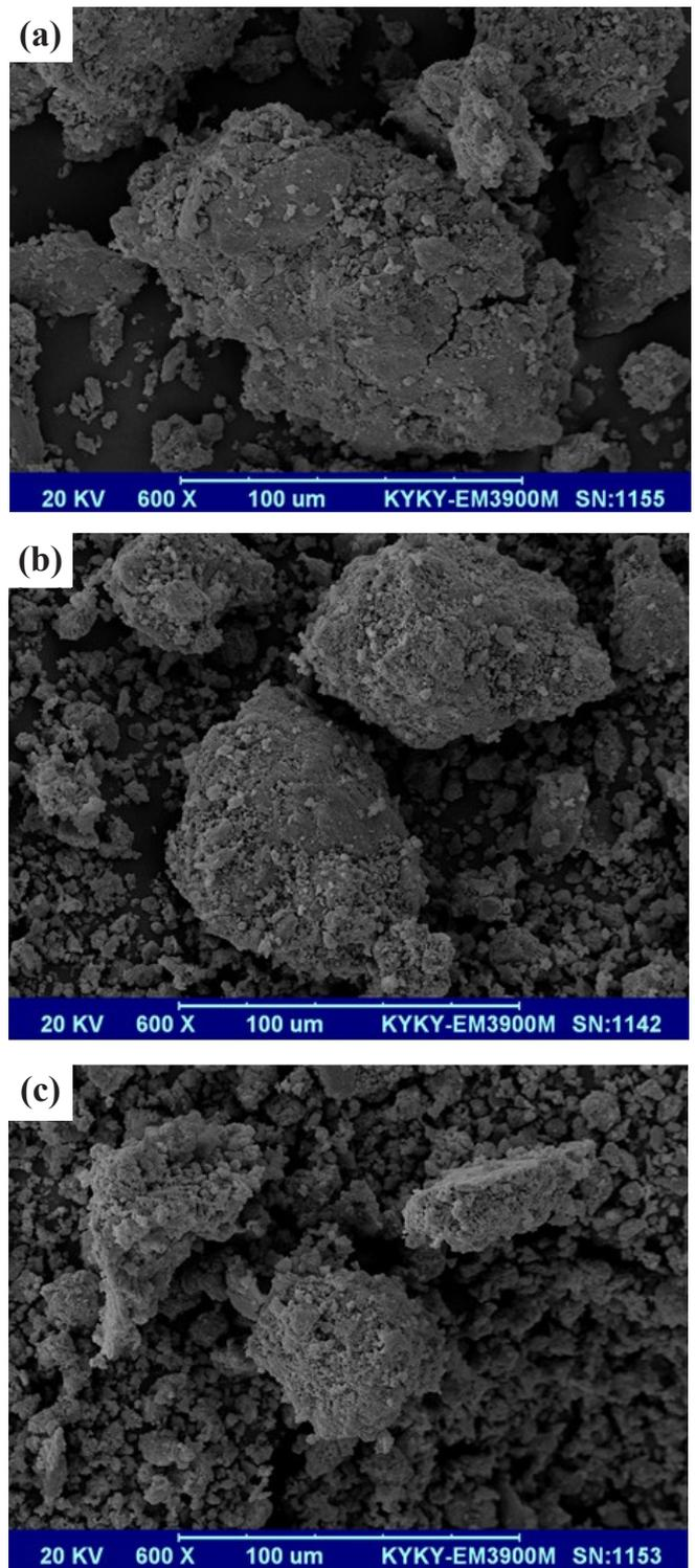
**Fig. 1.** The SEM micrograph of the Al-5% ZrSiO<sub>4</sub> powders after (a) 3 h, (b) 6 h, and (c) 9 h of ball milling.
