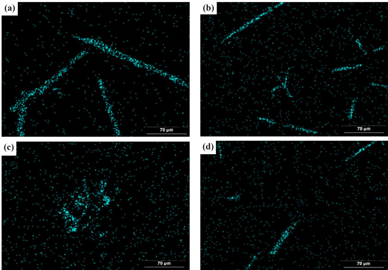
**Fig. 2.** (a),(c) The x-Ray map of Zr distribution in the matrix of the A356-( $ZrSiO_4$ )<sub>p</sub> composite and (b),(d) the A356-( $Al-ZrSiO_4$ )<sub>cp</sub> composite with the casting method of (a),(b) LL and (c),(d) SL.
