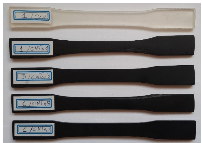
Fig. 3. The prepared samples for tension testing.
