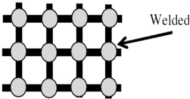
Fig. 2. Illustration of welded points in SRPE pipes [13].
