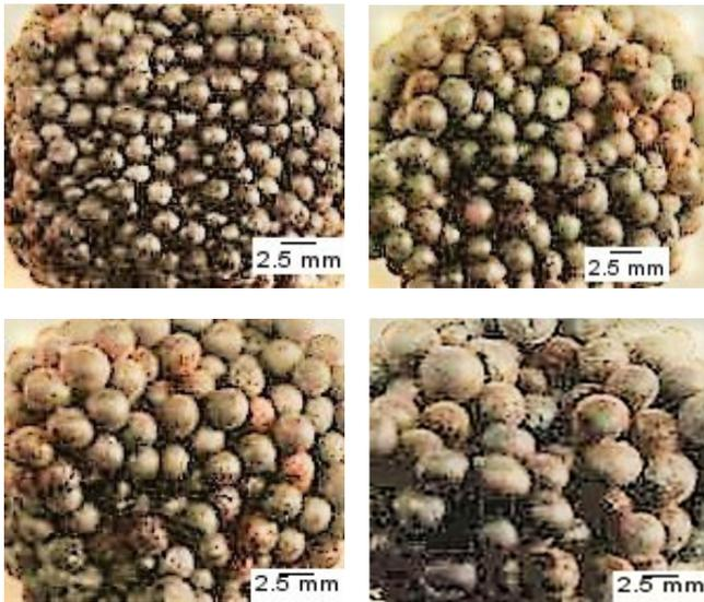
Fig. 2. Optical images of the sintered steel particles with different size preforms.
