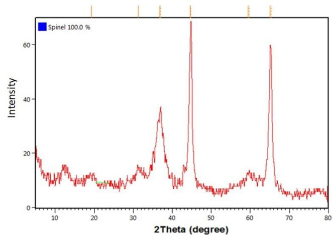
Fig. 4. XRD pattern of a sample synthesized and post-heated at 700 °C for 3 h.
