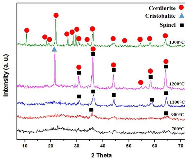
Fig. 8. XRD patterns of compacts of the mixture of activated synthesized magnesium aluminate and silica powders post-heated at different temperatures for 3 h.
