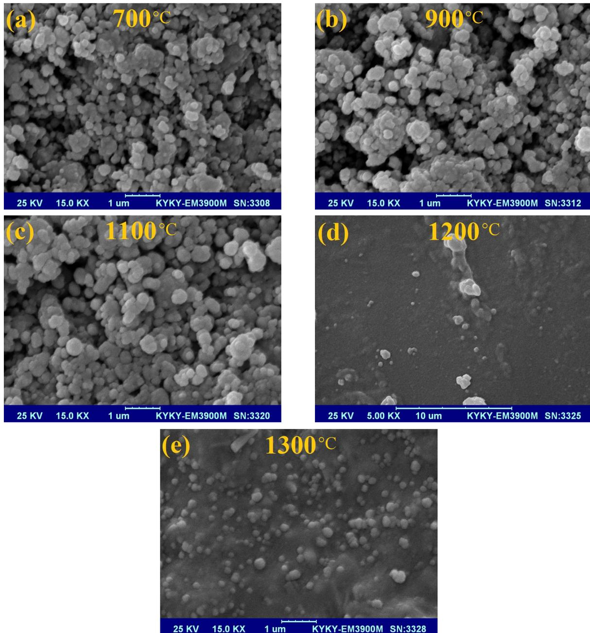
**Fig. 10.** SEM micrographs of compacts of the mixture of activated synthesized magnesium aluminate and nanosilica powders post-heated at (a) 700 °C, (b) 900 °C, (c) 1100 °C, (d) 1200 °C, and (e) 1300 °C.
