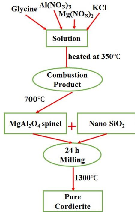
Fig. 3. Flowchart of cordierite synthesis.
