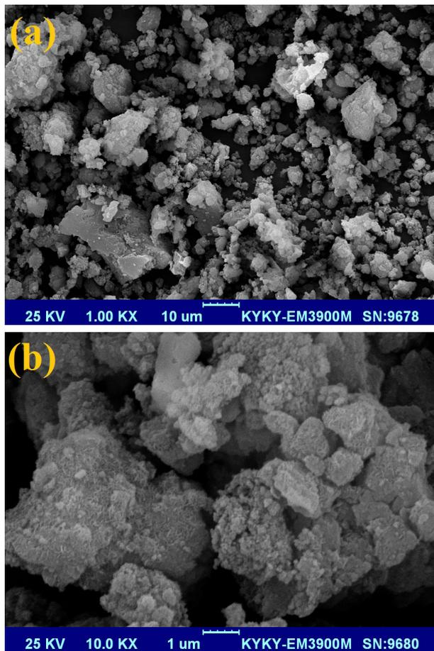
**Fig. 5.** SEM micrographs of magnesium aluminate spinel particles synthesized and post-heated at 700 °C for 3 h at different magnifications.
