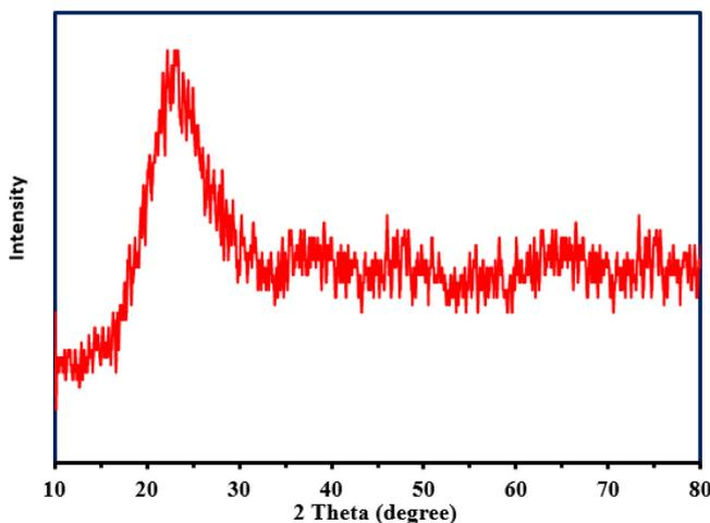
Fig. 2. XRD pattern of nanosilica purchased from Fadak Knowledge based Corporation.
