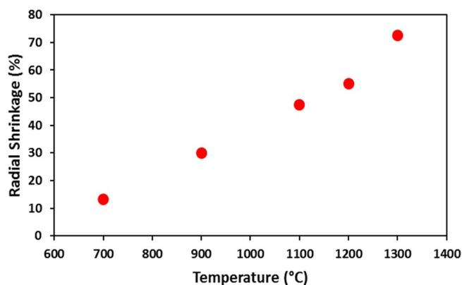
**Fig. 11.** Radial shrinkage (%) of compacts of the mixture in activated synthesized magnesium aluminate and nano silica powders post-heated at different temperatures.
