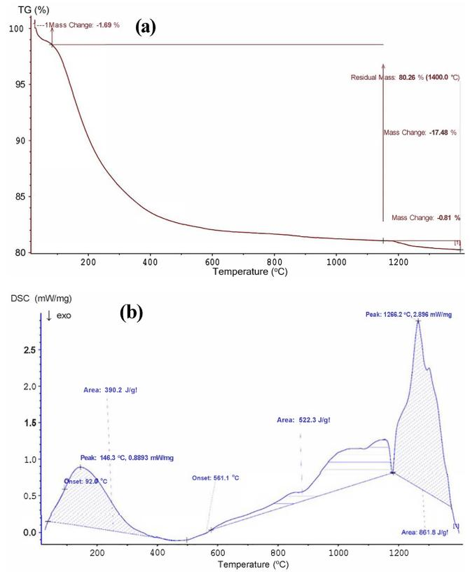
Fig. 9. Simultaneous thermal analyses (STA) of the mixtures of synthesized magnesium aluminate and silica powder activated by milling for 24 h (a) TGA and (b) DSC.
