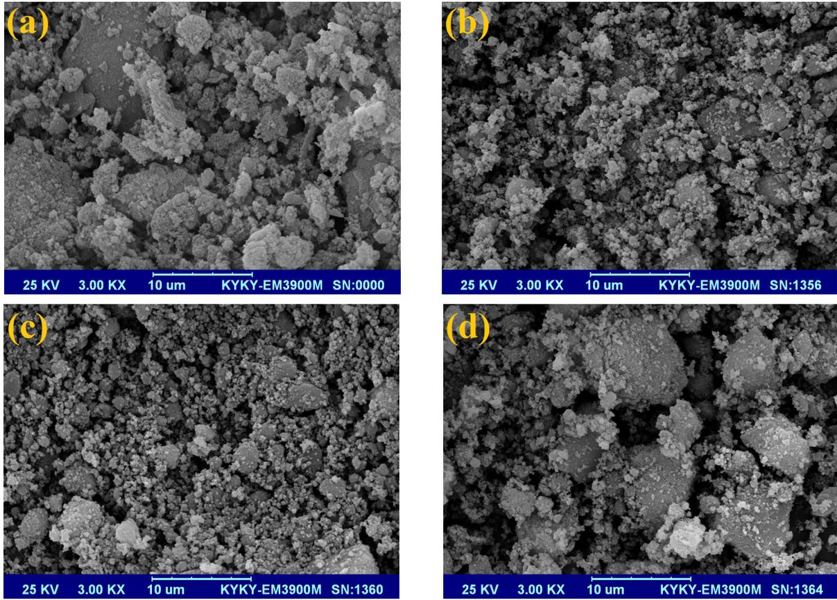
Fig. 7. SEM micrographs of mixtures of magnesium aluminate spinel and silica powders milled for (a) 5 min, (b) 6 h, (c) 18 h, and (d) 24 h.
