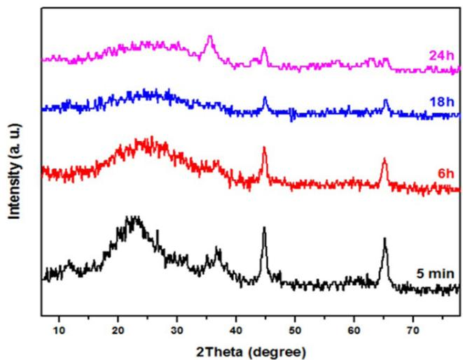
**Fig. 6.** XRD patterns of mixtures of magnesium aluminate spinel and silica powders planetary milled for different intervals.
