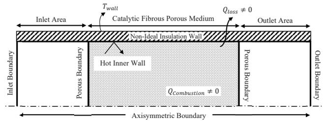
Fig. 5. The computational domain with assigned boundary conditions based on [20].
