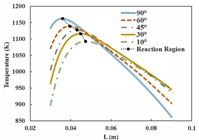
Fig. 6. Temperature distributions on the reactor's center line for five different fiber orientations at constant porosity.
