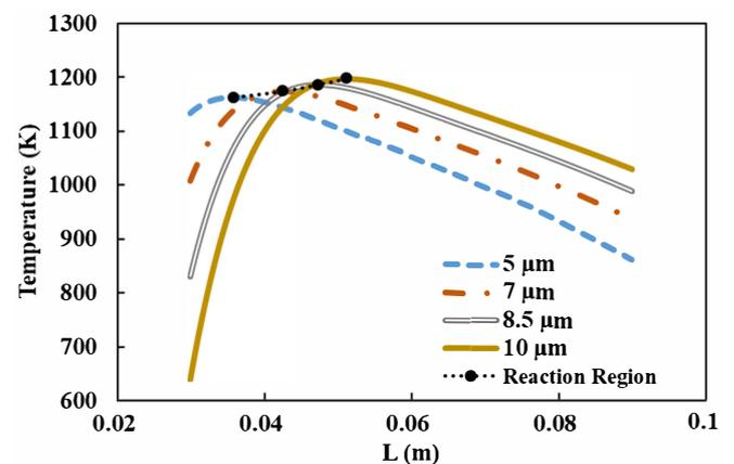
Fig. 8. Temperature distribution on the reactor's center line for four fiber diameters, 5, 7, 8.5, and  $10\ \mu\text{m}$ , in the constant porosity of the porous medium.
