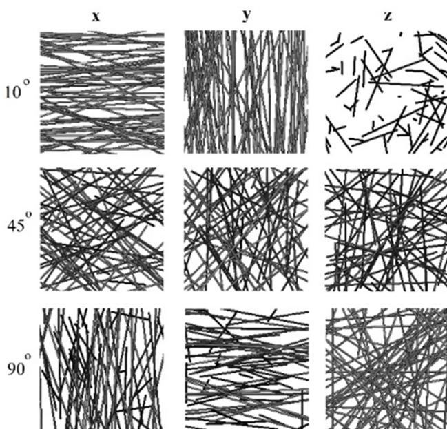
**Fig. 2.** The fiber's orientation in the fibrous medium for three different angles of  $10^\circ$ ,  $45^\circ$ , and  $90^\circ$  [22].
