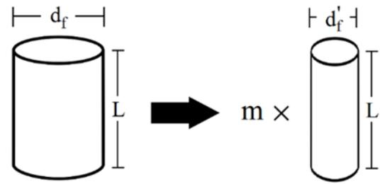
**Fig. 3.** Converting a fiber to  $m$  fibers of the same length at constant porosity [22].
