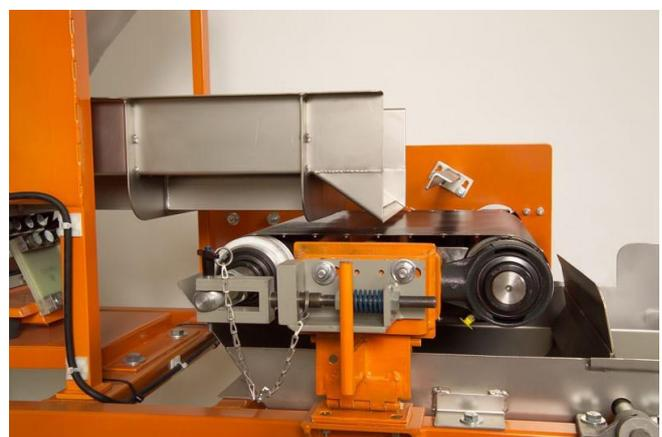
**Fig. 4.** Eriez rare earth roll, magnetic separator in Central Metallurgical Research and Development Institute.
