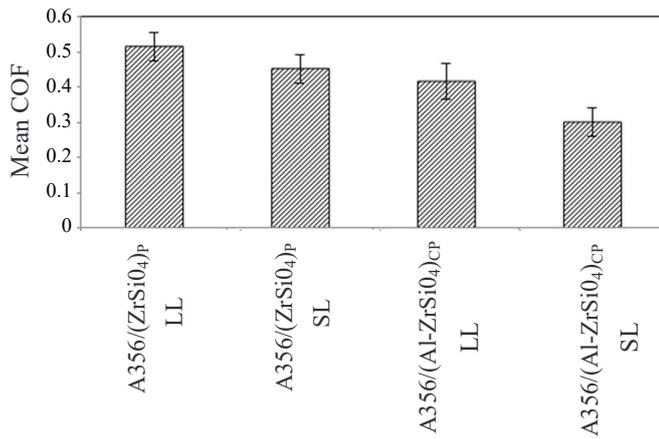
Fig. 5. The variations of the mean COF of the fabricated specimens.
