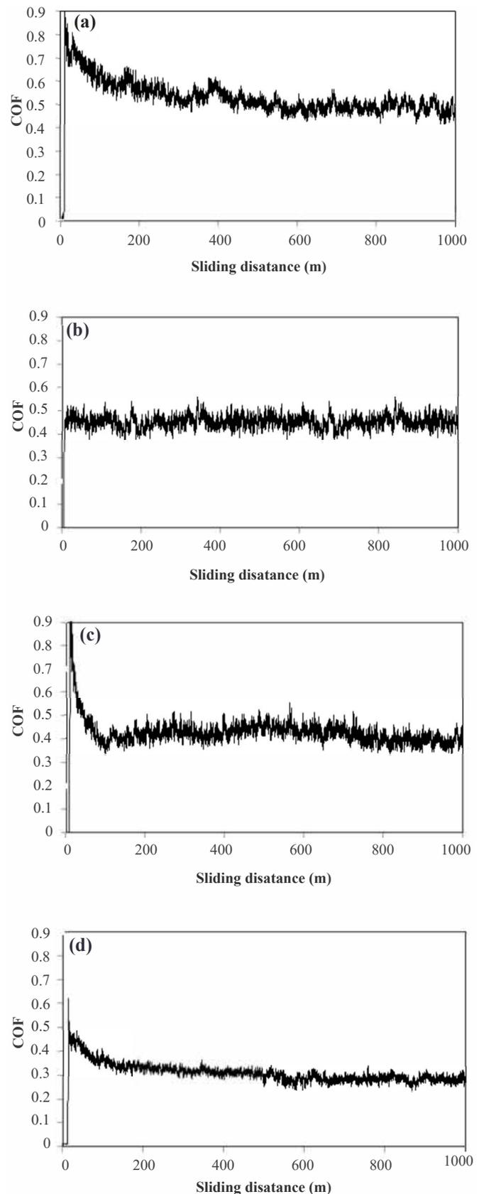
Fig. 4. The COF-sliding distance curves for the fabricated specimens (a) A356/(ZrSiO<sub>4</sub>)<sub>p</sub>-LL, (b) A356/(ZrSiO<sub>4</sub>)<sub>p</sub>-SL, (c) A356/(ZrSiO<sub>4</sub>)<sub>cp</sub>-LL, and (d) A356/(Al-ZrSiO<sub>4</sub>)<sub>cp</sub>-SL.
