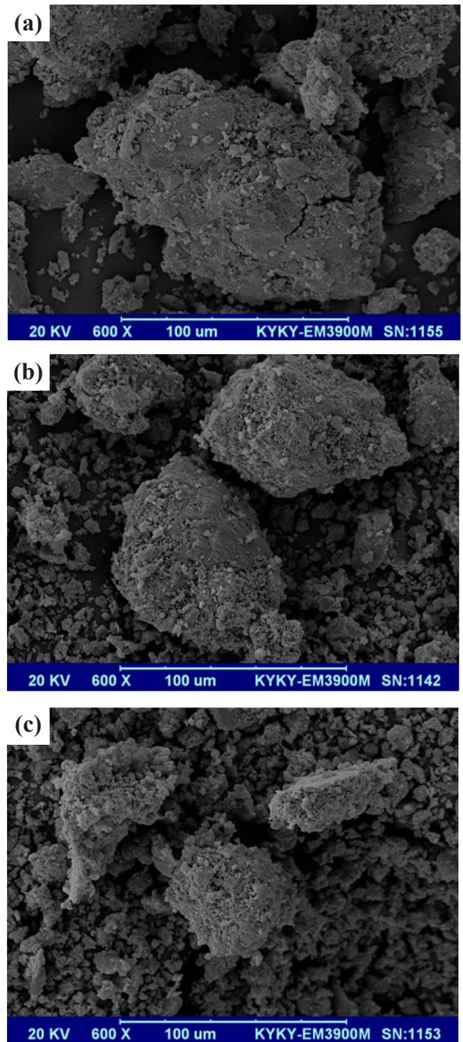
Fig. 1. The SEM micrograph of the Al-5%  $ZrSiO_4$  powders after (a) 3 h, (b) 6 h, and (c) 9 h of ball milling.
