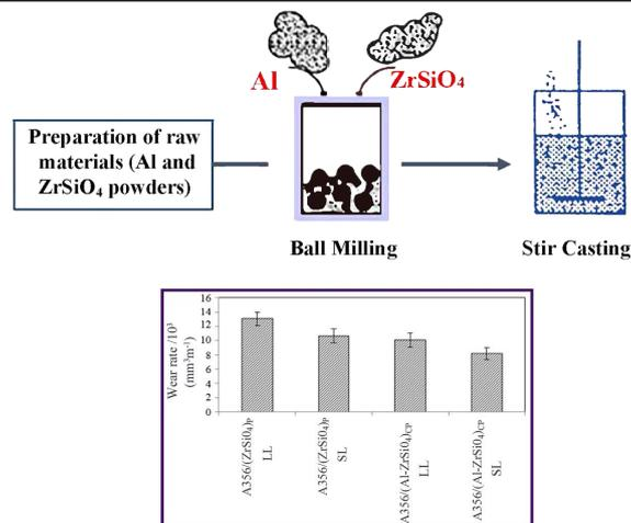
Wear rate of the fabricated composites
