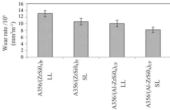
Fig. 3. The variations of the wear rate of the fabricated specimens.
