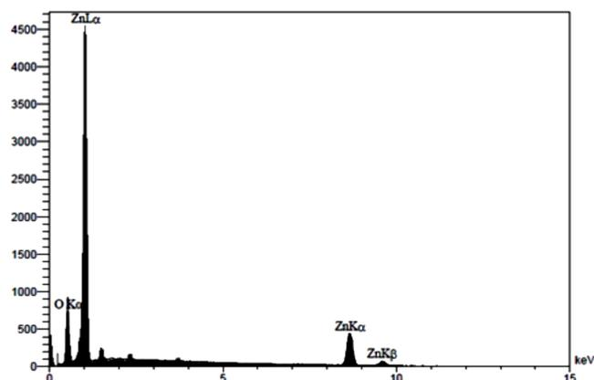
Fig. 11. Energy-dispersive X-ray analysis of hexagonal ZnO particles.
