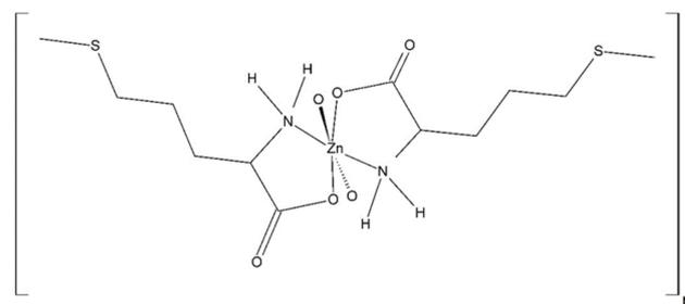
Fig. 2. The molecular structure of Zn-Meth complexes.
