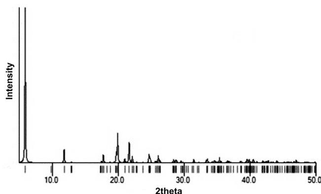
Fig. 5. XRD pattern of crystal Zn-Meth.
