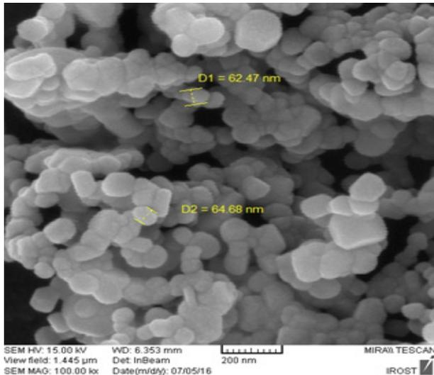
Fig. 12. SEM photograph of ZnO Nanoparticles.
