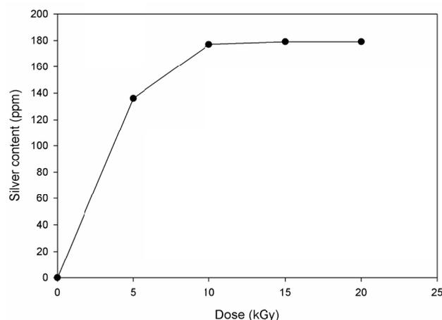
**Fig. 1.** Relationship between the content of AgNPs on the silk fabrics and irradiation dose.
