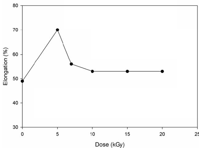
**Fig. 3.** Effect of different irradiation dose on the elongation (%) at break of untreated silk fabric and AgNPs-treated silk fabrics with different gamma irradiation doses.
