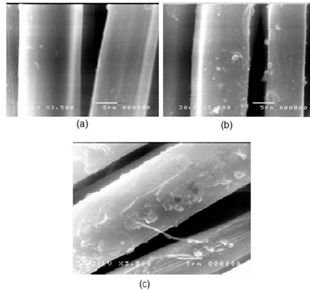
**Fig. 4.** SEM of untreated and AgNPs-treated silk fabrics with different gamma irradiation doses, a) Original silk fabric, b) 5 kGy, c) 10 kGy.
