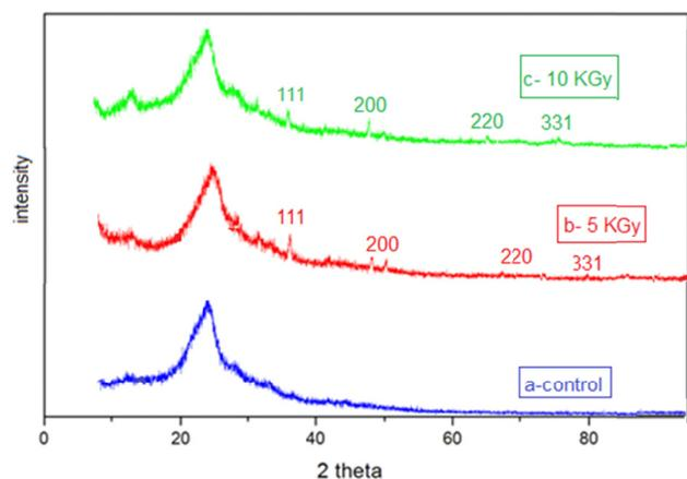
**Fig. 5.** XRD patterns of untreated (a) and AgNPs-treated silk fabric with different gamma irradiation doses (b and c).
