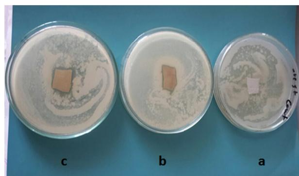
**Fig. 7.** Antibacterial effects of the untreated and AgNPs-treated silk fabrics on *E.coli* (A) Gram-negative bacteria.
