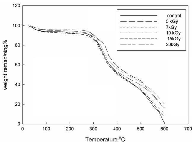
**Fig. 6.** TGA curves of untreated and AgNPs-treated silk fabric with different gamma irradiation doses.
