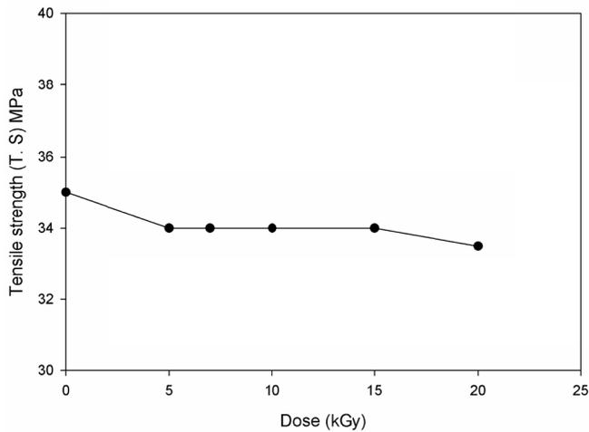
**Fig. 2.** Effect of different irradiation dose on the tensile strength at break of untreated silk fabric and AgNPs-treated ones with different gamma irradiation doses.
