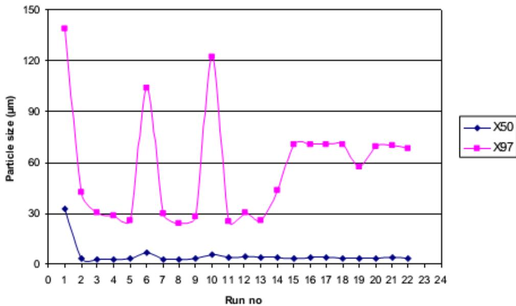
**Fig. 2.** Particle size (X<sub>50</sub> and X<sub>97</sub>) of the feed sample and products
