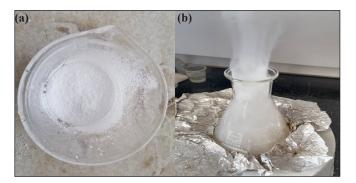
Fig. 1. Macro-image of (a) synthesized spinel powders and (b) combustion.
