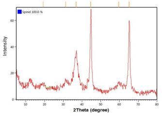
Fig. 4. XRD pattern of a sample synthesized and post-heated at 700  $^{\circ}$ C for 3 h.
