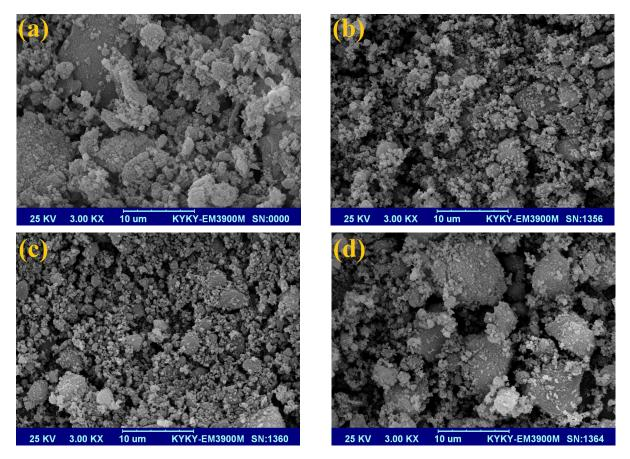
Fig. 7. SEM micrographs of mixtures of magnesium aluminate spinel and silica powders milled for (a) 5 min, (b) 6 h, (c) 18 h, and (d) 24 h.
