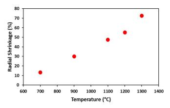
**Fig. 11.** Radial shrinkage (%) of compacts of the mixture in activated synthesized magnesium aluminate and nano silica powders postheated at different temperatures.
