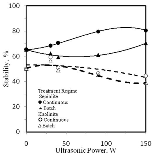
Fig. 5. The effect of the treatment regime of ultrasonic on the stability of clay suspensions.
