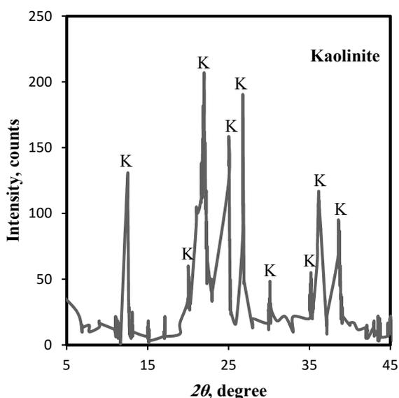
Fig. 1. X-ray diffraction pattern of the clay samples.
