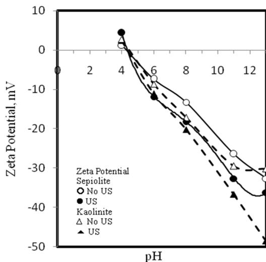
**Fig. 3.** The effect of ultrasonic treatment on the zeta potential of clays at different pH values.
