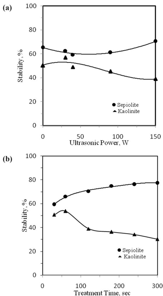
**Fig. 4.** The stability of clay suspensions depending on (a) ultrasound power and (b) treatment time.
