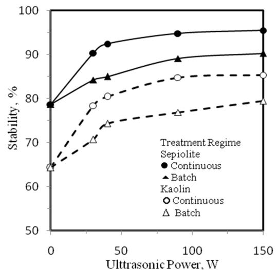
Fig. 7. The effect of the treatment regime of ultrasound on the dispersion of clay suspensions.
