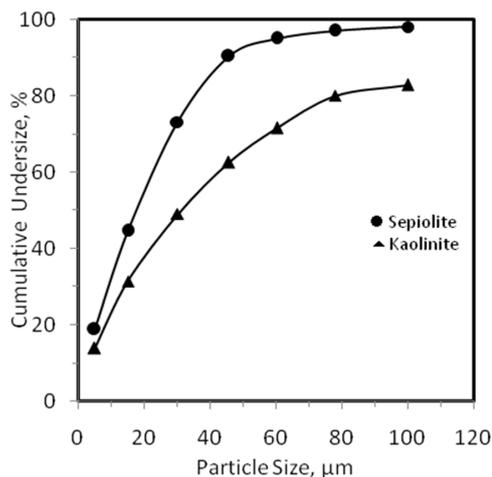
Fig. 2. The particle size distribution of the clay samples used in the experiments.
