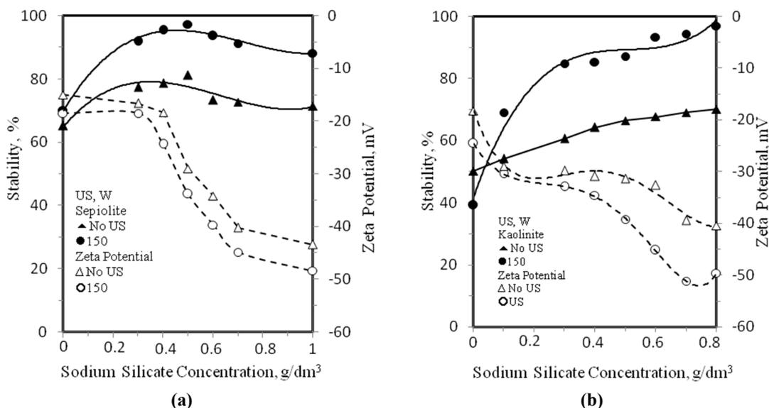
Fig. 8. The effect of ultrasonic process on the dispersion and zeta potential of clays depending on sodium silicate concentration.
