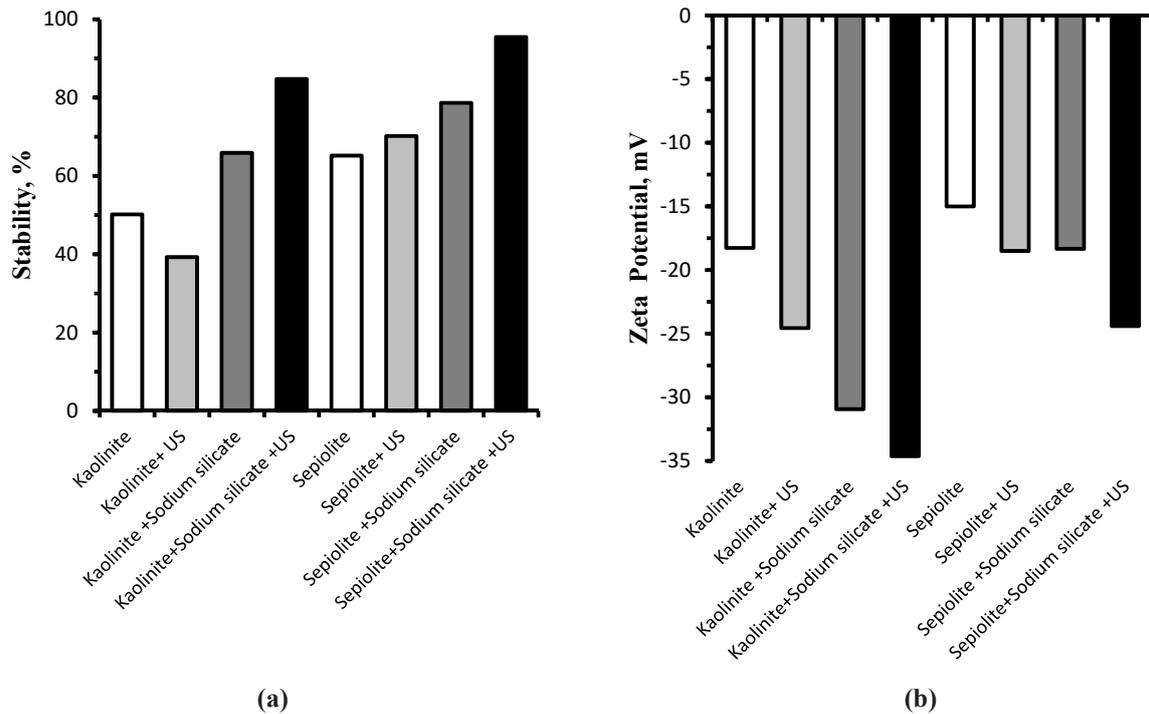
**Fig. 9.** The effect of ultrasonic treatment on the (a) suspension stability and (b) zeta potential of clays.
