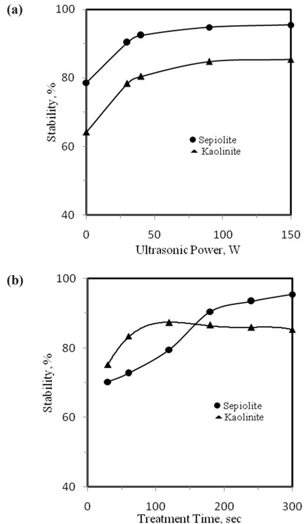
Fig. 6. The effect of (a) ultrasonic power and (b) treatment time on the dispersion of clay suspensions.
