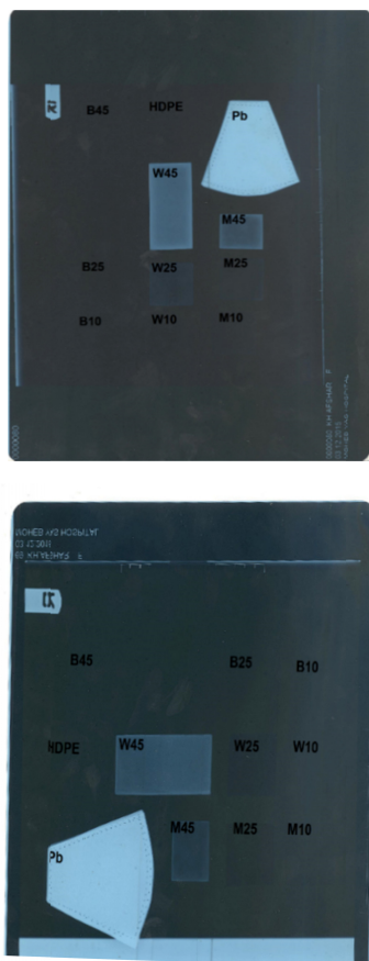
Fig. 3. Radiology images at intensities of a) 40 and b) 80 KeV x-ray for neat lead, 10 and 45 % (wt) of boron carbide, tungsten and molybdenum disulfide in HDPE.
