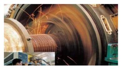
Fig. 8. The welding machine of metallic wires (square morphology).
