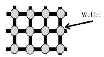
Fig. 2. Illustration of welded points in SRPE pipes [13].
