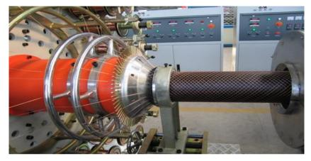
**Fig. 7.** Unit of wire winding of the reinforced polyethylene composite pipes in Goldstone Orient New Material Equipment Company, China.
