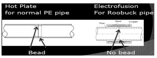
Fig. 3. Electrofusion welding is used in steel wire reinforced HDPE pipes and un-reinforced ones [17].
