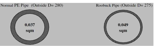
Fig. 1. Comparing flow area of SRPE with usual PE pipes produced in Roobuck factory.
